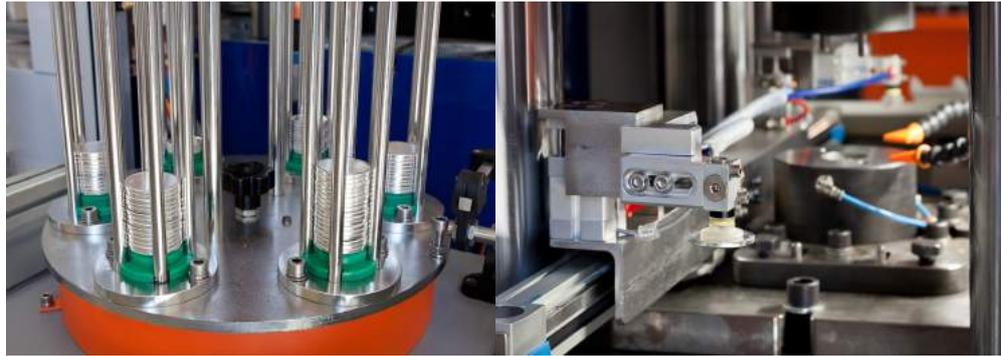
Standard feeding system from the 6-fold blanks magazine located at the side of the press, the blanks are taken by vacuum cups and placed to the coining tool.
